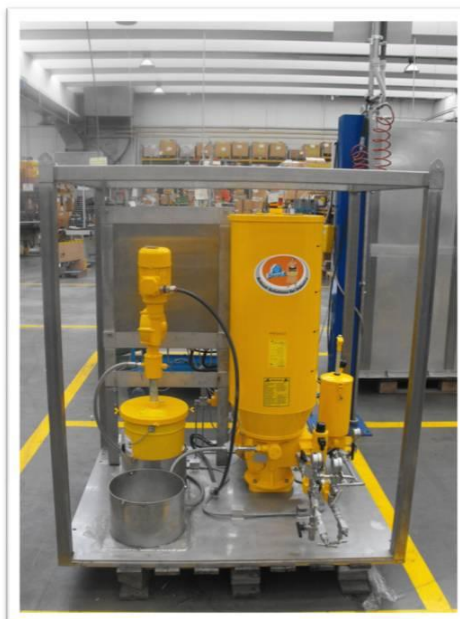
SUMO 100kg Pump with custom yellow coating assembled on a custom Stainless 316 Skid assembly incorporating a PLC control system Manual back up pump and electric barrel pump for filling
