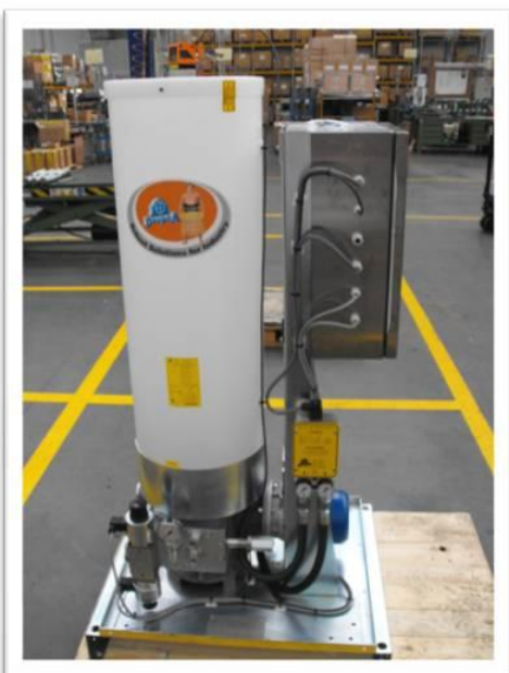
SUMO Pump semi-transparent reservoir with end of line pressure switches and control panel in a stainless box installed on the standard pallet
