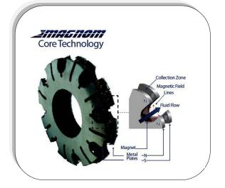
Magnom<sup>™</sup> core elements are comprised of an annular magnet and two innovatively formed steel plates. The steel plates direct the lubricant flow and magnetic flux through channels designed to bring all the ferrous contaminants in the lubricant within the range of the magnets.
