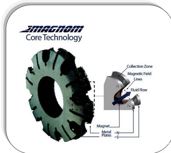
Magnom™ core elements are comprised of an annular magnet and two innovatively formed steel plates. The steel plates direct the lubricant flow and magnetic flux through channels designed to bring all the ferrous contaminants in the lubricant within the range of the magnets.
