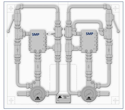
The SMP units are fitting with the latest Dropsa Ultrasensor spool sensor product: a revolutionary patented system that has no moving parts and made in AISI 316 Stainless Steel.
